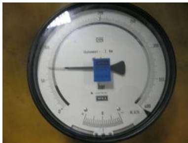
manometer at P=69bar for the first 3 steps
