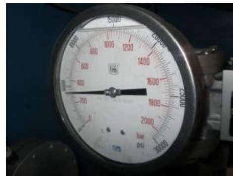
P=280bar constant for 2 minutes and pressure arousal until burst occurs
