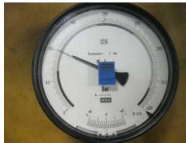
manometer at P=103bar for the second 3 steps
