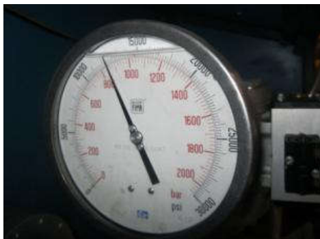
P=280bar constant for 2 minutes and pressure arousal until burst occurs
